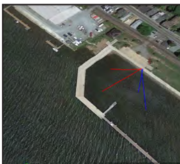
Figure 74 One system aeration concept of four airlines and two compressors to address odors and algae in the jetty area using solar power. One system would create improvement, but a double system would be needed for complete coverage of the whole area inside the pier
